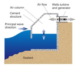
b) An oscillating water column (OWC) [4, 5, 6]
