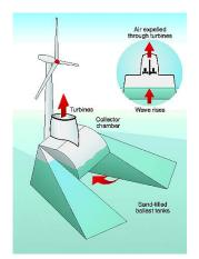
a) Wave-powered electricity generator [3]
