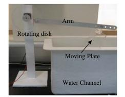
(b) The wave generator is to produce ripples in the water surface resulting in waves
