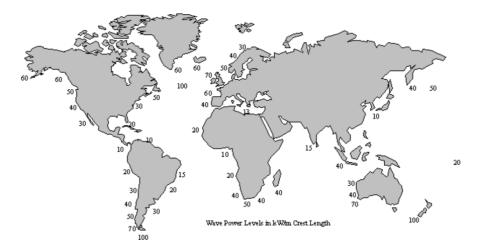
Figure 2. Approximate global distribution of time-average deep water wave power in kW/m of wave front [2].
