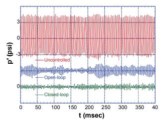
Figure 1. Comparison of uncontrolled and controlled pressure oscillation amplitudes [2].
