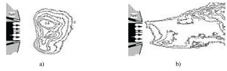
Figure 2. Actively controlled diffusion flames, a) efficient and b) sooty flames [3].
