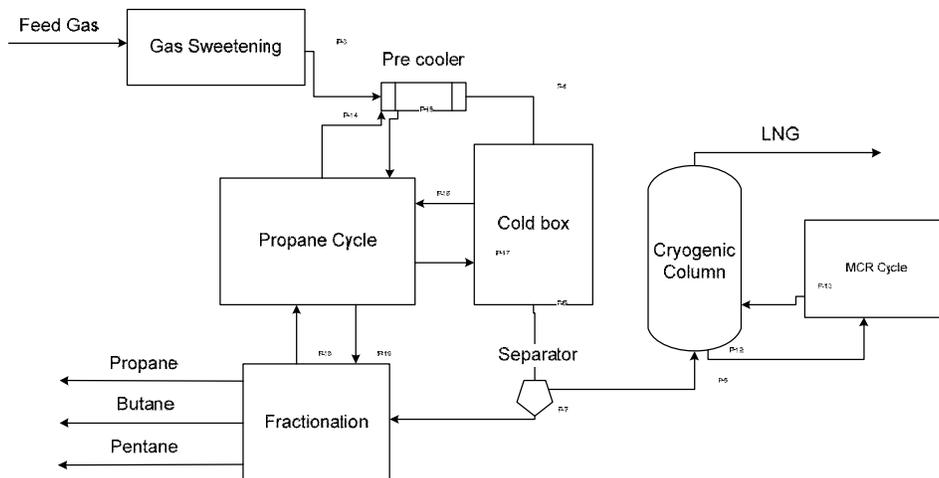
Figure 2. Schematic illustration of an LNG plant-process.
