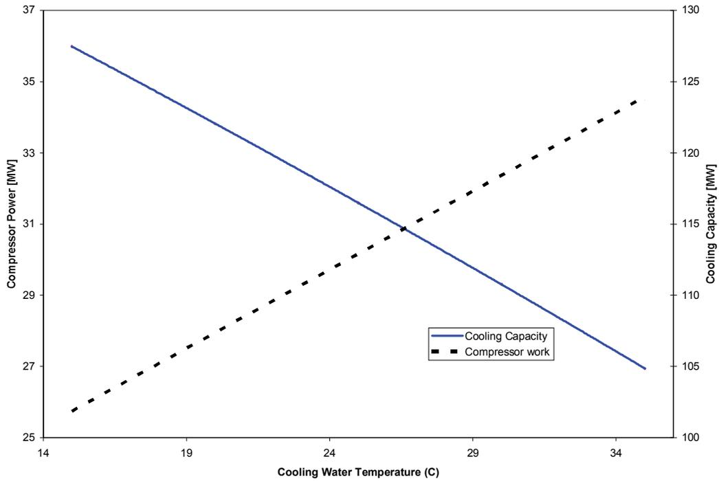
Figure 9. Predicted effect of cooling water temperature on total cooling capacity and compressor power.
