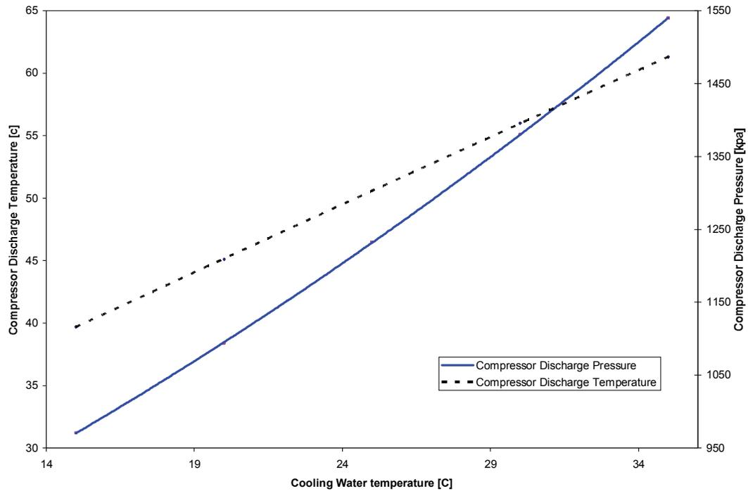
Figure 10. Predicted effects of cooling water temperature on compressor discharge pressure and temperature.
