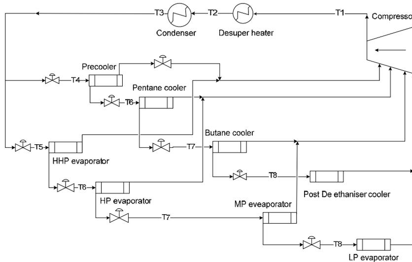
Figure 6. Propane cycle block diagram.
